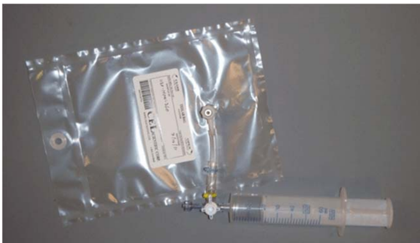
Figure 7-8: One-liter Tedlar Bag with Disposable Syringe and Three-way Valve for Filling.
