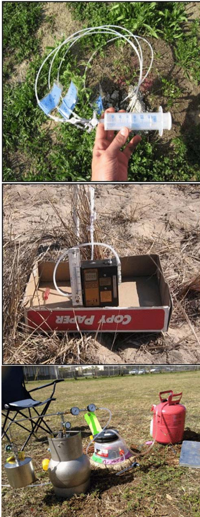
Figure 7-31: Soil Vapor Probe Purging Devices Upper photo: Disposable syringe with 3-way Luer valve (see also Figure 7-26 ). Middle photo: Pump with flow meter. Lower photo: Large Summa used for purging. Smaller Summa to left used to collect sample after purging; purge Summa closed during sample collection
