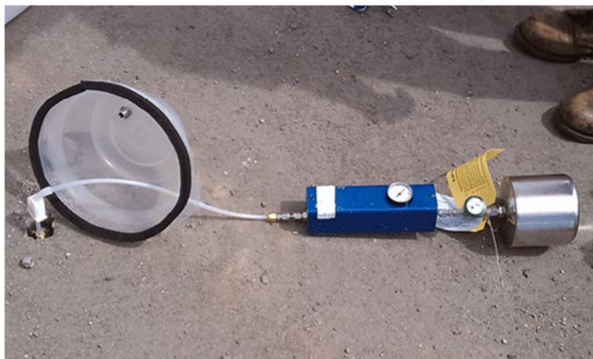
Figure 7-34: Summa canister sampling trains. Upper schematic: Diagram of Summa canister soil vapor sampling apparatus. Lower photo: Teflon tubing connected to flow controller with Swagelok and to well point with short length of flexible tubing (allowed well point to be closed for followup sorbent tube sample). Note Tupperware shroud used for leak test.
