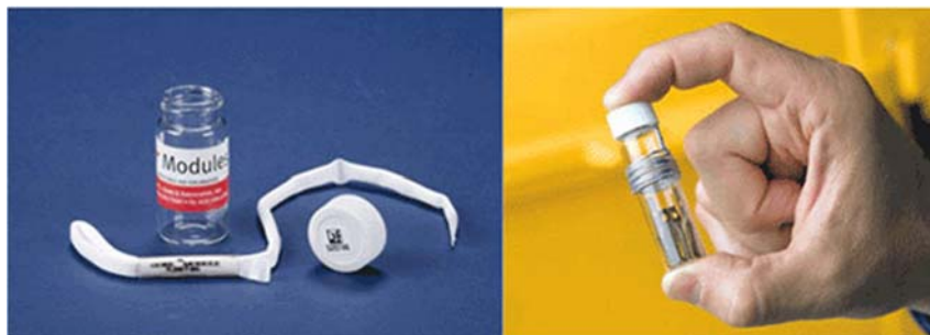
Figure 7-10 Two Examples of Passive Soil Vapor Sample Collectors.
