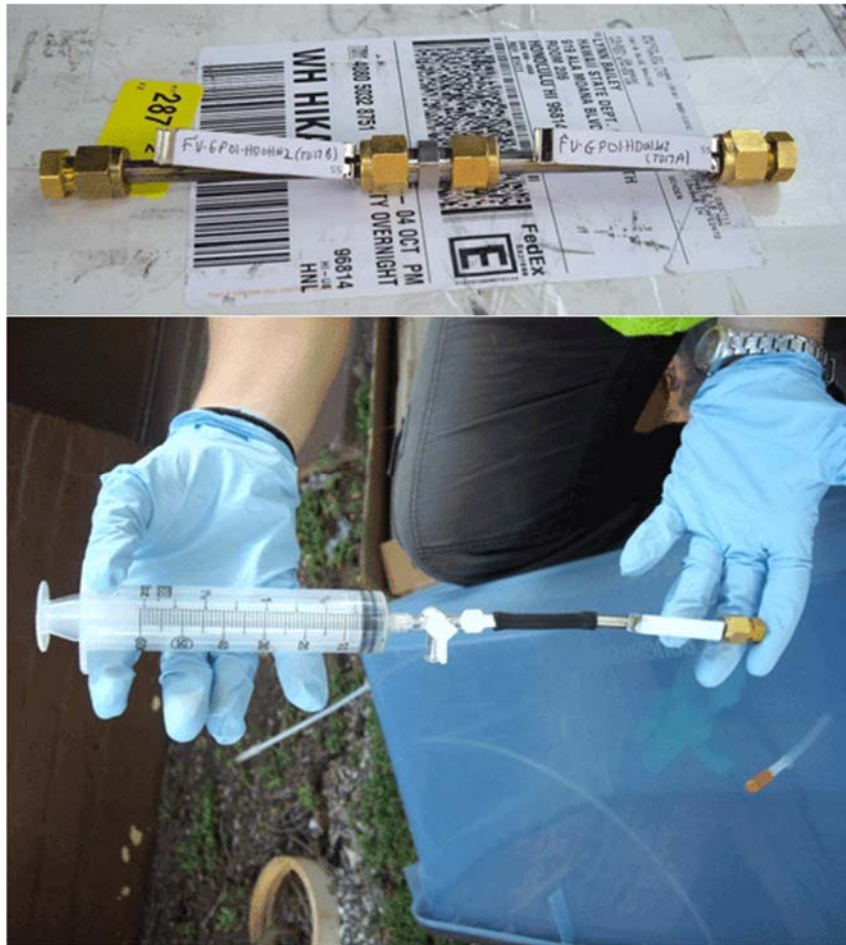
Figure 7-9: Sorbent Tubes. Upper photo: Sorbent tubes connected in series with a union fitting. Lower photo: Single sorbent tube connected to a 60ml syringe for collection of vapor sample (see also Figure 7-27 ).
