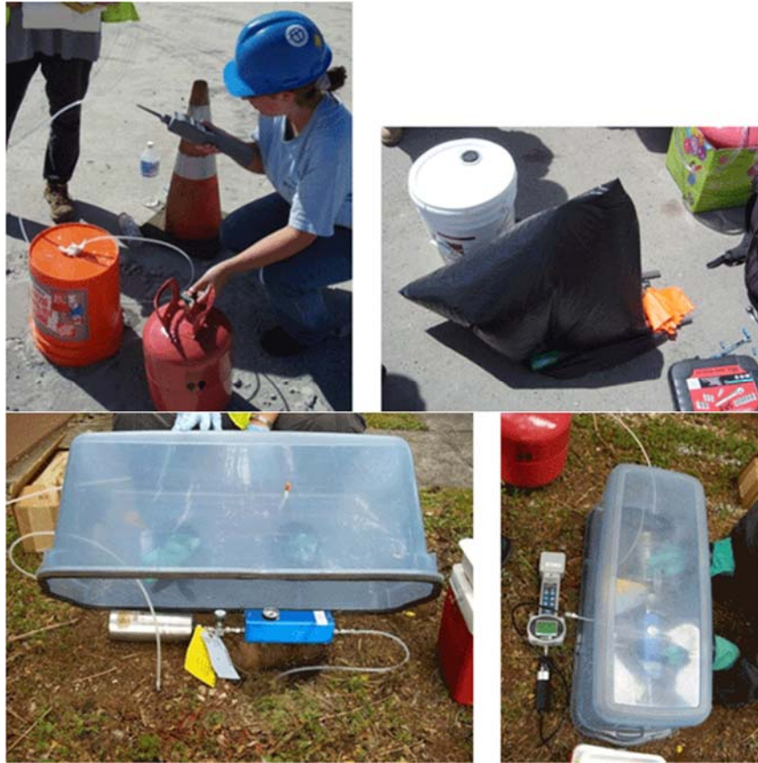
Figure 7-39: Method 2 Helium Shroud Leak Testing Systems Helium released into shroud and used as tracer to identify leaks in both sampling train and vapor probe annular seal. Upper left photo: Five-gallon bucket helium shroud placed over well point and Summa canister-flow controller sampling train (note two ports for injection and monitoring of helium inside shroud). Upper right photo: Use of garbage bag as shroud (helium injected under shroud to fill bag). Lower photos: Large Tupperware container converted to shroud, with fill ports for helium injection and monitoring, plus glove ports to open and close Summa canister for sample collection.
