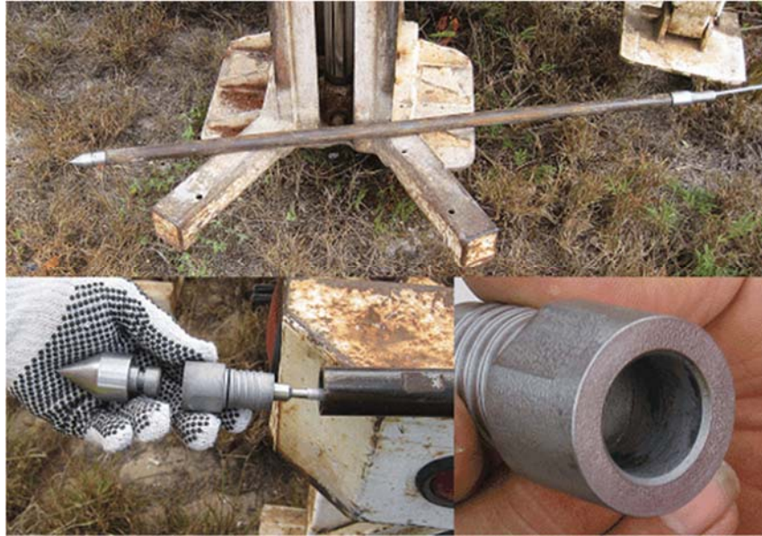
Figure 7-22: Typical Temporary Soil Vapor Probe Typical temporary soil vapor probe, designed to be driven by a direct-push drill rig. The probe tip components (from left to right in the lower left photo) include a disposable drop-off point, probe tip (threaded to attach the tip to a steel drill rod), inert tubing connecting the probe tip to a sampling pump on the surface, and a steel drill rod. A fine mesh screen is located inside the probe tip.
