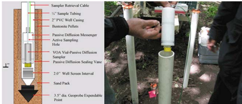
Figure 7-12: Passive Diffusion Sampler (PDS). Schematic of sampler on left and photo of a sampler being installed on the right.
