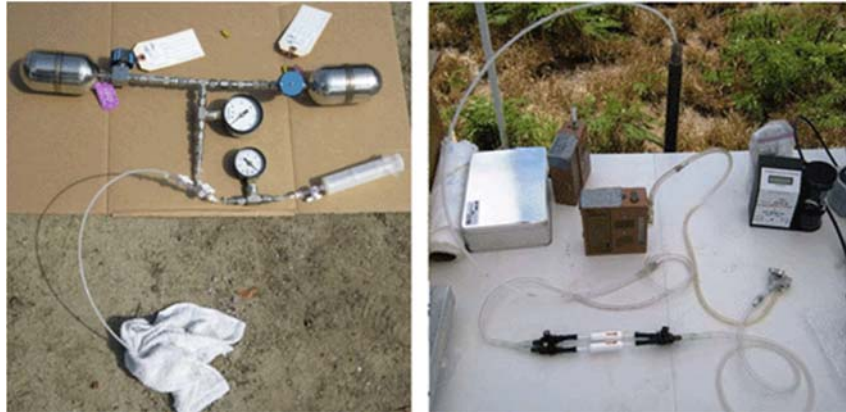
Figure 7-43: Typical Duplicate Sampling Apparatus (see also Figure 7-35 ). Left photo: Stainless steel "T" manifold to simultaneously collect primary and duplicate soil vapor samples in 500-ml Summa canisters. Right photo: Laboratory-supplied duplicate sampling apparatus to simultaneously collect primary and duplicate soil vapor samples in sorbent tubes.
