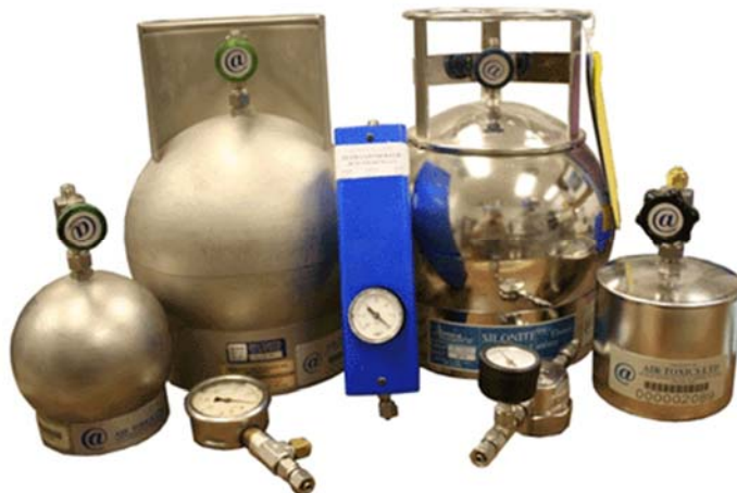
Figure 7-5 Summa Canisters (spherical and cylindrical containers) with Flow Controllers (smaller gauges and blue box).
