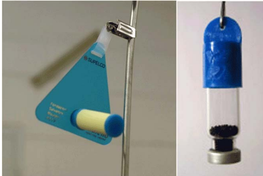
Figure 7-11: Two Examples of Indoor Air Passive Sample Collectors.
