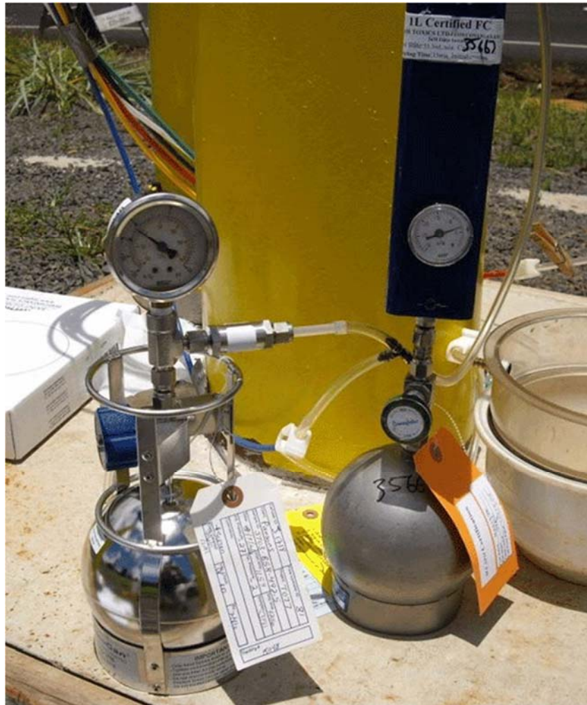
Figure 7-6 Summa Canister and Flow Controller Setups (note smaller flow controller on left).
