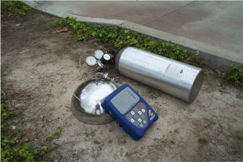
Figure 7-21: Schematic Diagram and Photograph of Flux Chamber
